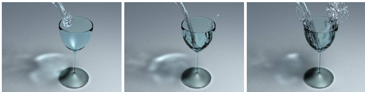
Figure 1. Example of an adaptive free surface simulation with the VOF LBM algorithm.
