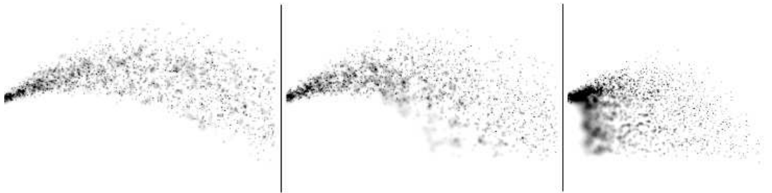
Figure 10.5: Effect of the drag model for different size scales. The simulations were parametrized to represent scales of 10cm, 1m and 10m, from left to right. The smaller particles, are slowed down, and cause mist below the outflow.
