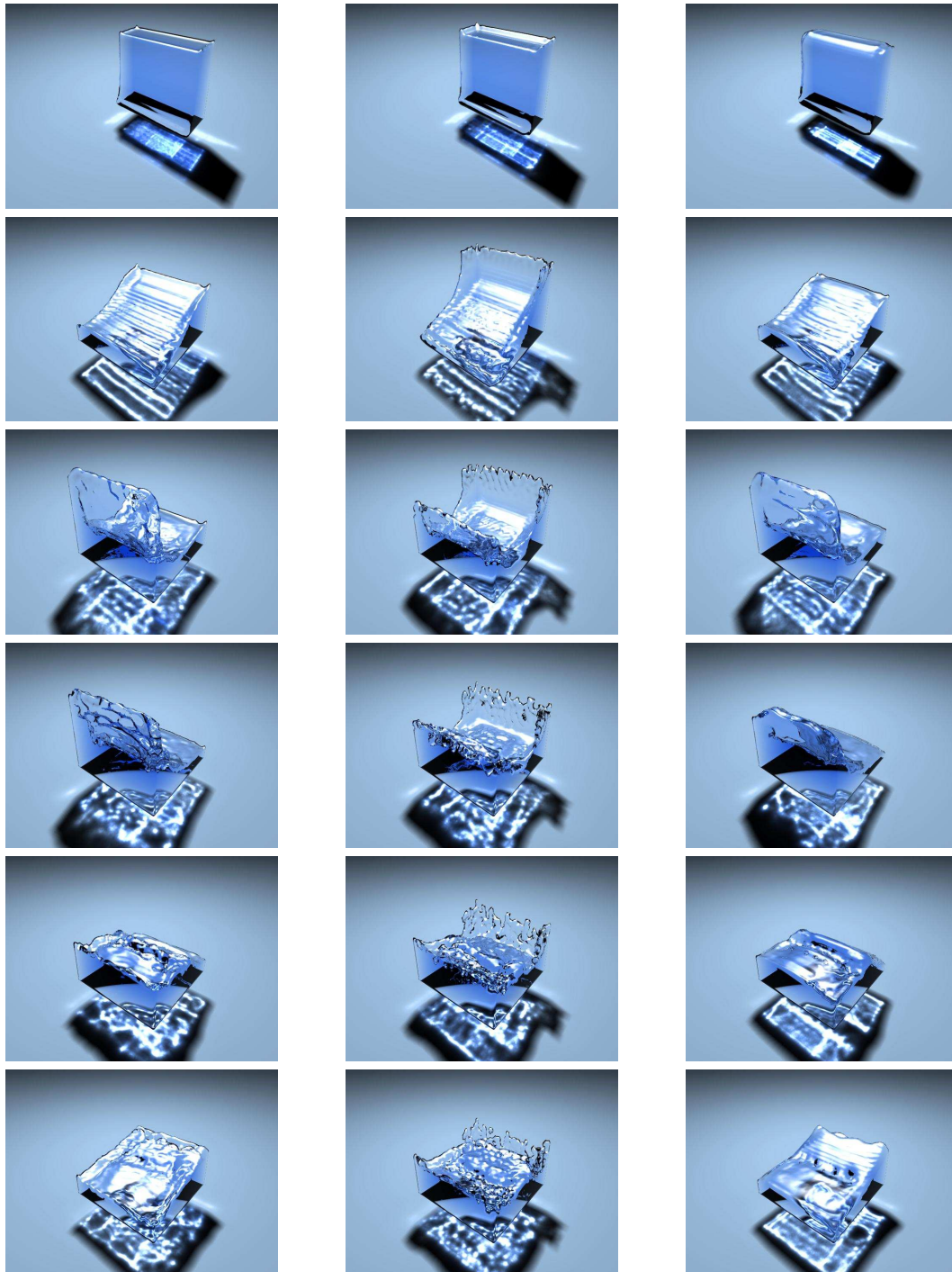
Figure 6.2: The standard breaking dam problem. To the left with free-slip boundary conditions, with no-slip walls in the middle and to the right with free-slip walls and surface tension.
